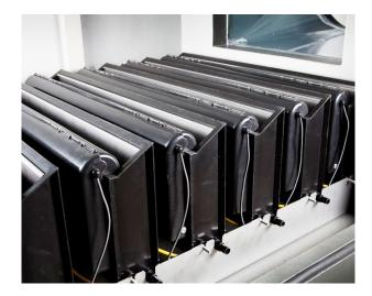
made to the air when it is inside the machine itself – which means that there is little to no fluctuation in the environmental conditions in the HatchTech MicroClimer Setters and Hatchers. Such stable and uniform environment is one of the key factors in achieving optimal and uniform chick quality.
